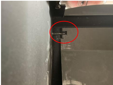
Firebrick correctly located on pin
